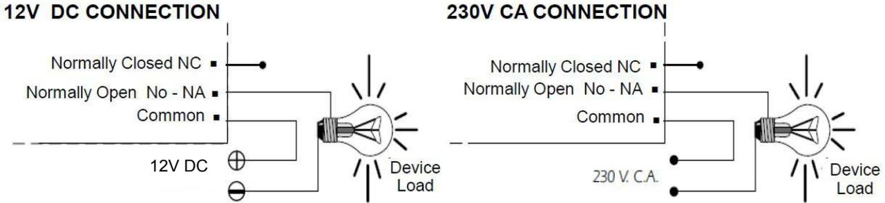
**CONSIDERATIONS ON THE RELAY.** Especially with inductive loads, a relay output can produce a fluctuation rate, or an incorrect operation. If this happens, install anti-spark circuit between the two relay contacts used in the connection, which will ensure the absorption of peak current that causes the above problem.
