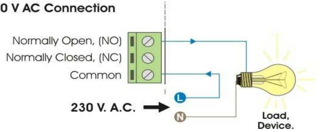
**INFORMATION ABOUT THE OUTPUT.** During the circuit operating mode and according to its load, it could happen a fluctuation or an incorrect working of the output. In such case, you have to install an anti-spark circuit between both contacts of the used relay, as it is indicated on the drawing.
