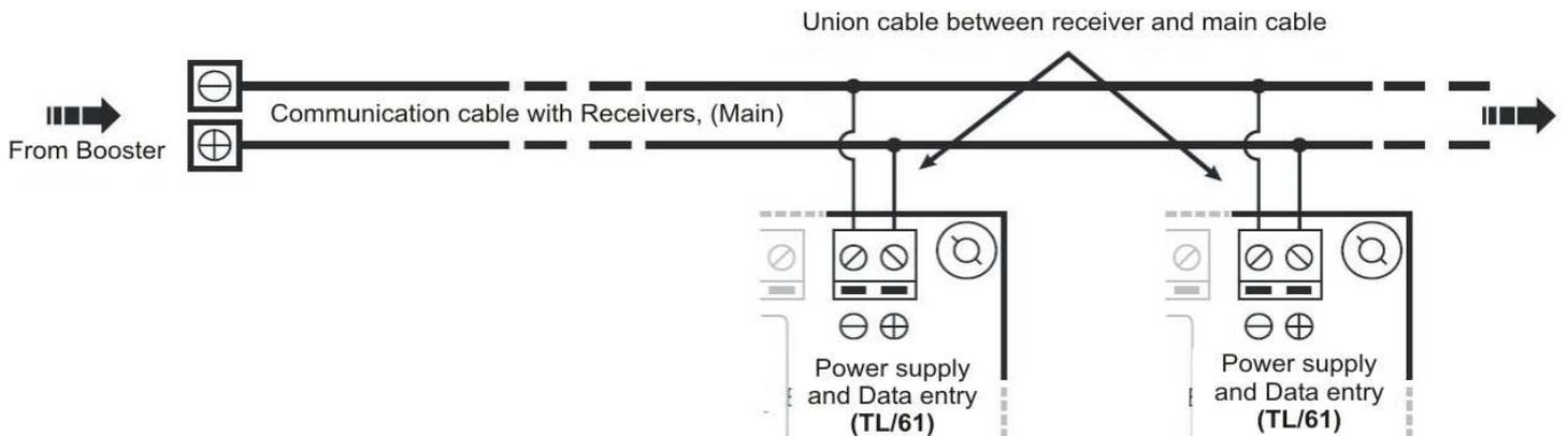
Therefore, connect the positive and the negative cables of the power supply input and Data of the TL-61 to the respective positive and negative Communication Cable with Receivers. Before to follow the installation, make sure that the assembly has been correctly done.
