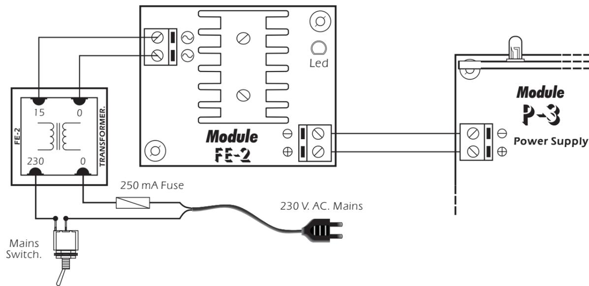
**OPERATING.** Once these connections done, you could supply the module. Then, automatically one of 4 included led will light on. On the P-3's front panel, you have a rotative switch with four different positions, corresponding to each channel of the module. According to the switch position, the module will inject to the output the selected input. The led corresponding to the selected channel will light on.
