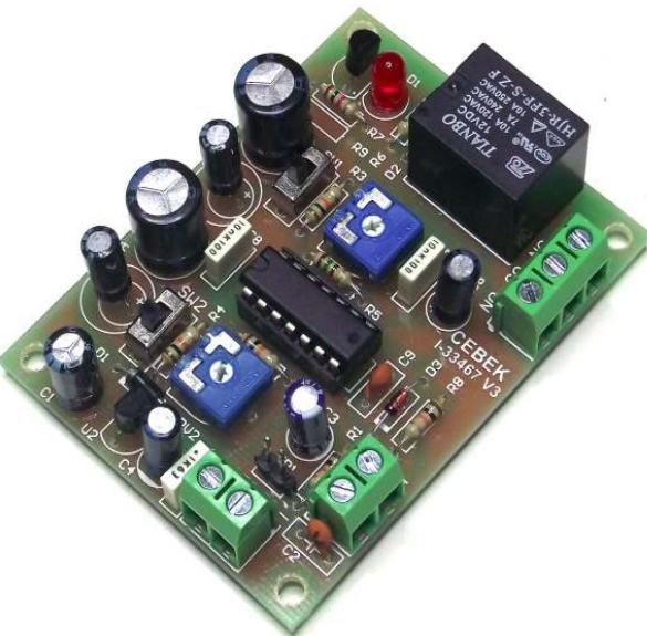
Timer with double time scale for ON and OFF using SW1 and SW2 (A or B scale), delay between 0,1 second and 4 minutes and triggering by push button or by power up. Pressing the Start button will initiate a pre-delay timing before relay connection. Once this has elapsed, the relay work timing will automatically be activated. The work led will light while the output is activated. Both Delay and Work times are independent of each other and adjustable through potentiometers RV1 and RV2.
