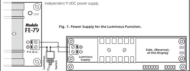
Fig. 7. Power Supply for the Luminous Function.
