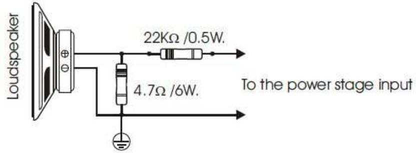
loudspeaker, install between the volume potentiometer and the loudspeaker following resistors according to the drawing hereafter.
