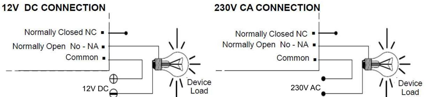
**ABOUT THE OUTPUT.** During operation of the circuit, and according to its load, it could happen a fluctuation or an incorrect output performance. If this happens, install a circuit sparking between the two relay contacts used in this connection, as shown in the drawing.
