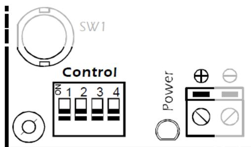
OPERATION. The DA-04 is an intelligent circuit, specially designed to control access to doors with an external ring. The module, after being recorded a tune in memory, and then connecting it to the doorbell, you'll see every keystroke made on it. If the pulses correspond to the reproduction of the prerecorded melody, the trigger circuit output, allowing the opening of the door. If the pulses do not respond to the pattern of the melody, the circuit denied access.
