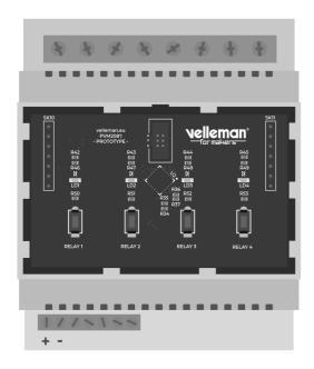
Step 2: plug the Ethernet cable into the module (at the bottom, right). Make sure that you can connect to the same network with another device. It can be a laptop or PC, Android device or iOS device.
