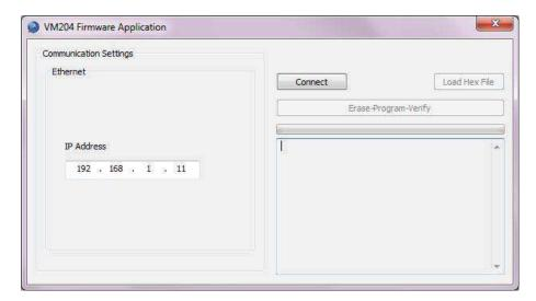
5. Hopefully you remembered your IP address! Copy it into the 'IP Address' field and press <Connect>. Normally, you should see 'device connected'.
