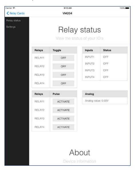
7. To edit your relay card, go back and slide over the name of your relay card to the left (for iOS) or long press the name of your relay card (for Android) and tap <Edit>.
