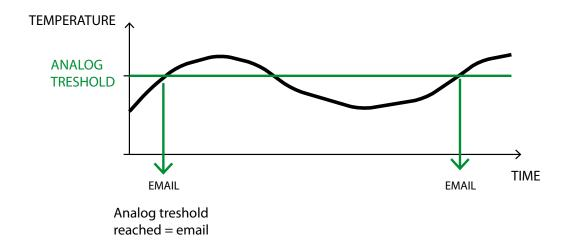
You can set the analog treshold value in the 'Alarm value' box after you select this action in the list (see picture below). The alarm value must be between 1 and 1024. This value can be calculated by multiplying your voltage value times 155. For example if your voltage value is 3.3 V then the calculation is: 3.3 V \* 155 = 511.5 => 512. Floating-point numbers are not valid so round your value up or down. The maximum voltage that can be sensed is 6.6 V (=1024).
