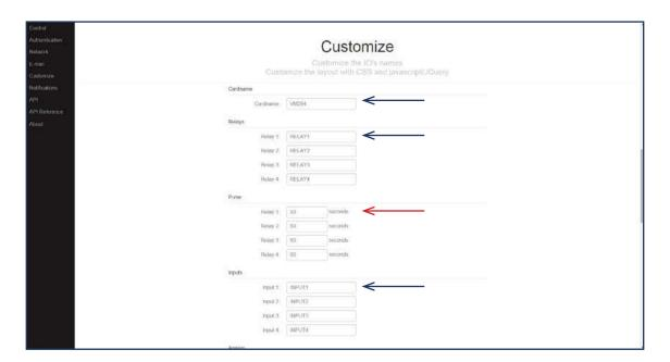
If you give each relay and input a different name, it's easy to remember what the relay is controlling or what the input is reading. For example 'lights bathroom' or 'doorbell'. These names will also be used when sending e-mails from the VM204.
