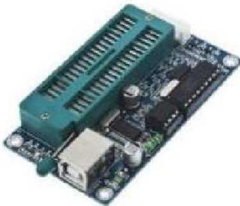
The AS3150ZIF is a USB Flash PIC® Microcontroller Programmer with ZIF programming socket and 6-pin ICSP connector. It is supplied fully assembled and ready to use with our free Windows programming software interface.
