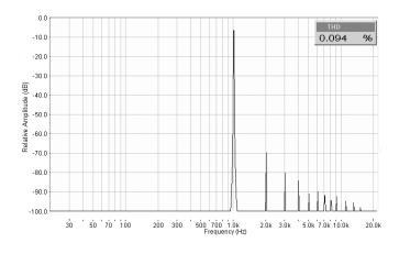
THD @ 1kHz, 1 Volt RMS output 8 Ohm Load
