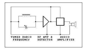
The second component of the TRF is the coil & ferrite bar. We supply the coil prewound with 90 turns of 3 strand Litz wire. We get these coils from a commercial manufacturer of these coils who supplies exactly the same item to AM radio manufacturers. Litz wire consists of many strands of fine enamelled wire twisted together with cotton to add strength. Litz wire has a significantly lower resistance to RF than a single wire and is used in virtually all commercial coils.
