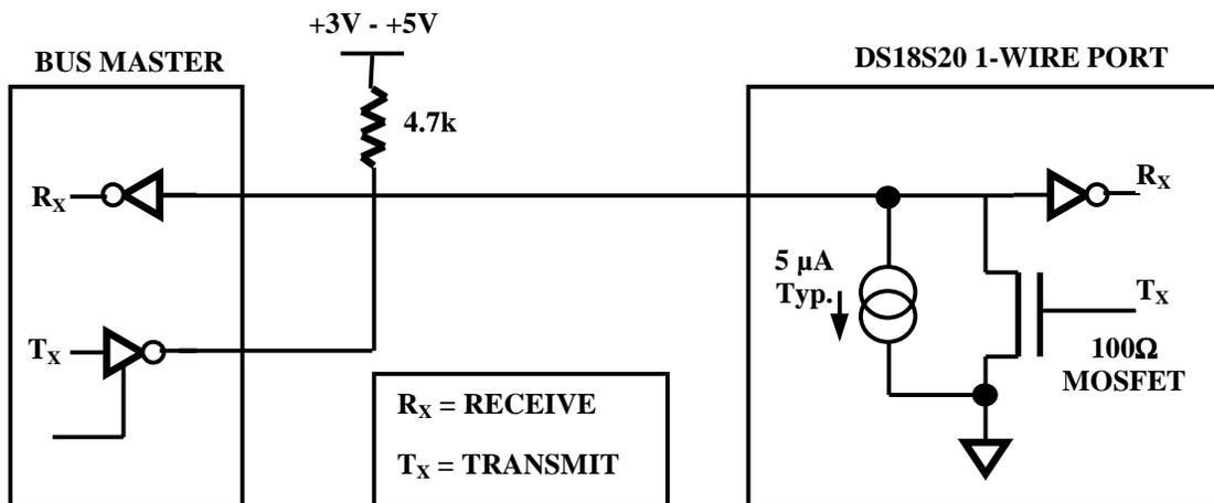
The idle state for the 1-Wire bus is high. If for any reason a transaction needs to be suspended, the bus **MUST** be left in the idle state if the transaction is to resume. Infinite recovery time can occur between bits so long as the 1-Wire bus is in the inactive (high) state during the recovery period. If this does not occur and the bus is left low for more than 480  $\mu\text{s}$ , all components on the bus will be reset.
